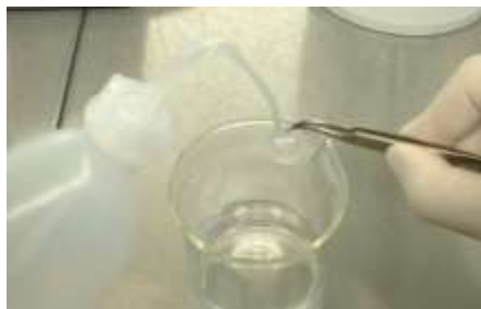
Figure 9: Rinsing: fill and empty 20 x
